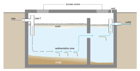
Figure 14 - Schematic diagram of septic tank
