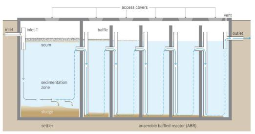
Figure 33 – Schematic diagram of ABR
