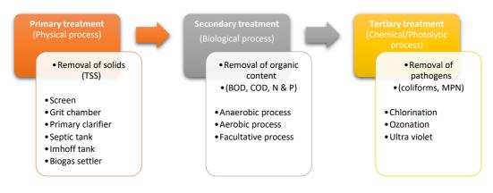
Figure 10 – Wastewater Treatment Chain
