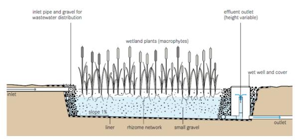
Figure 22 – Schematic diagram of horizontal flow constructed wetlands
