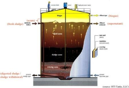
Figure 43 – Schematic diagram of Anaerobic Digestor
