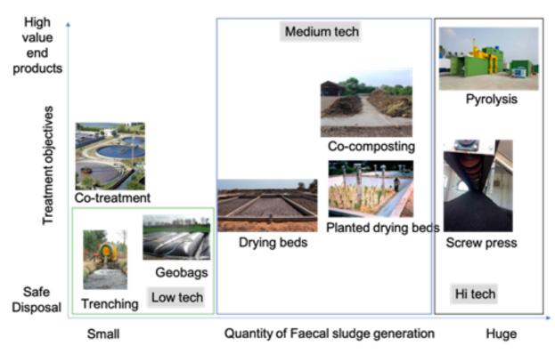
Figure 58 – Selection of treatment approach for Faecal Sludge/Septage
