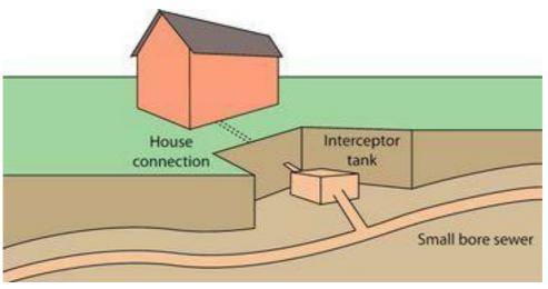
Figure 8 – Schematic diagram of small bore sewer system
