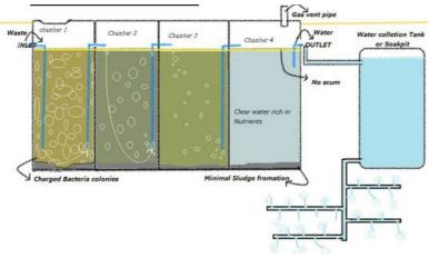
Figure 32 – Bio-digestor tank system
