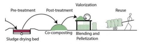
Figure 54 – Schematic diagram of Co-composting
