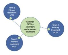
Figure 56 – Planetary Model
