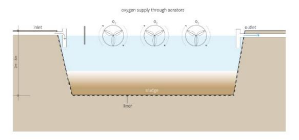
Figure 23 – Schematic diagram of aerated pond
