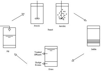
Figure 20 – Schematic diagram of SBR
