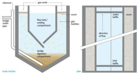
Figure 15 - Schematic diagram of Imhoff tank
