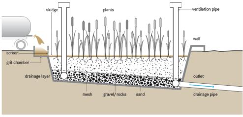
Figure 47 – Schematic diagram of Planted Drying Beds
