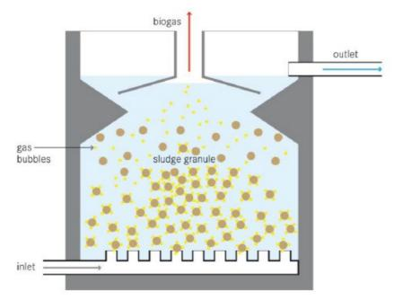
Figure 18 – Schematic diagram of UASB
