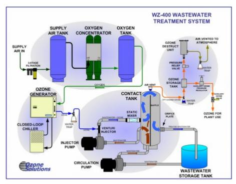
Figure 25 – Schematic diagram of Ozonation
