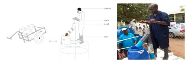
Figure 35 – Human powered emptying of OSS- Gulper
