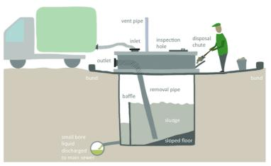
Figure 39 – Fixed type transfer station
