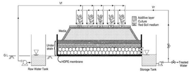
Figure 27 – Schematic diagram of SBT
