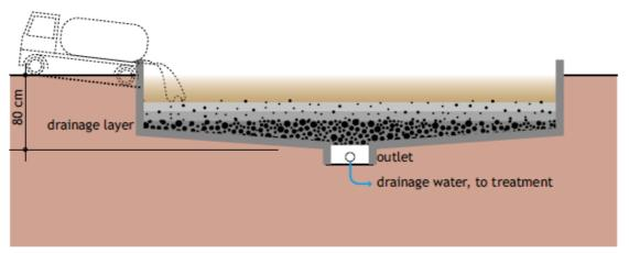
Figure 46 – Schematic diagram of Unplanted Drying Beds
