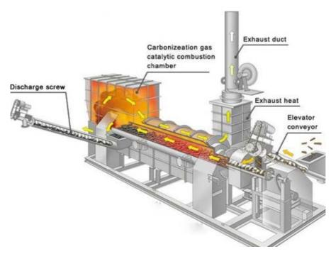
Figure 51 – Schematic diagram of Sludge Incineration Plant
