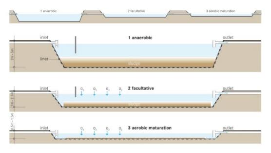
Figure 17 – Schematic diagram of WSP
