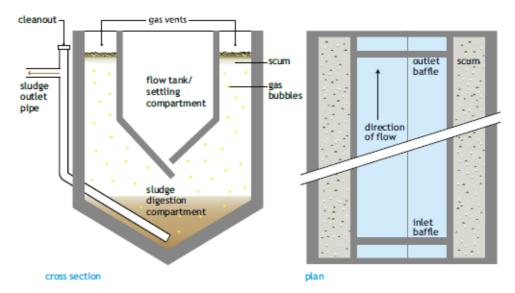
Figure 44 – Schematic diagram of Imhoff Tank
