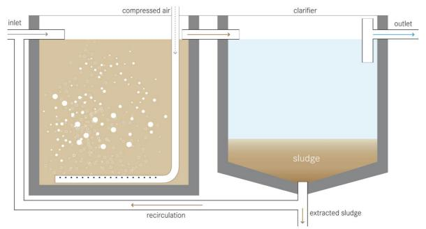
Figure 19 – Schematic diagram of ASP
