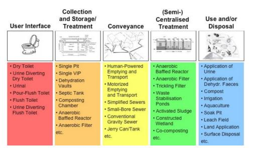
Figure 4 – Main Processing Systems of Sanitation
