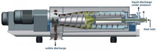
Figure 48 – Schematic diagram of Centrifuge
