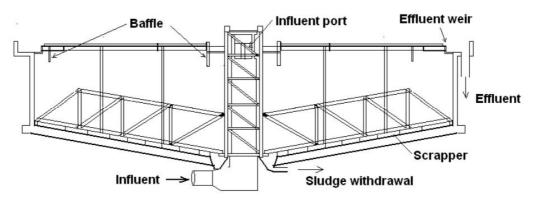
Figure 13 - Schematic diagram of primary clarifier
