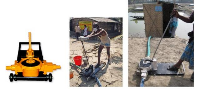
Figure 36 – Manually operated Diaphragm pump
