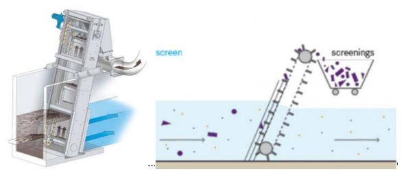
Figure 11 - Schematic diagram of screens
