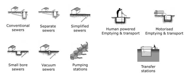
Figure 7 – Sewered Conveyance Options
