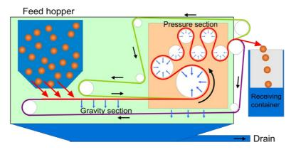
Figure 50 – Schematic diagram of Belt Press
