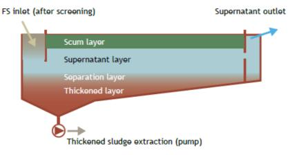
Figure 45 – Representative diagram of Settling – Thickening Tank
